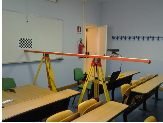
Fig. 3.33: The installation used to perform the shift tests varying the distance.
