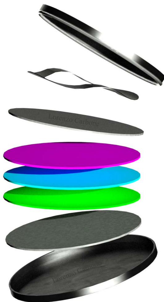
Scheme of the 2032-coin cell. Pink cathode, azure separator and green anode.
