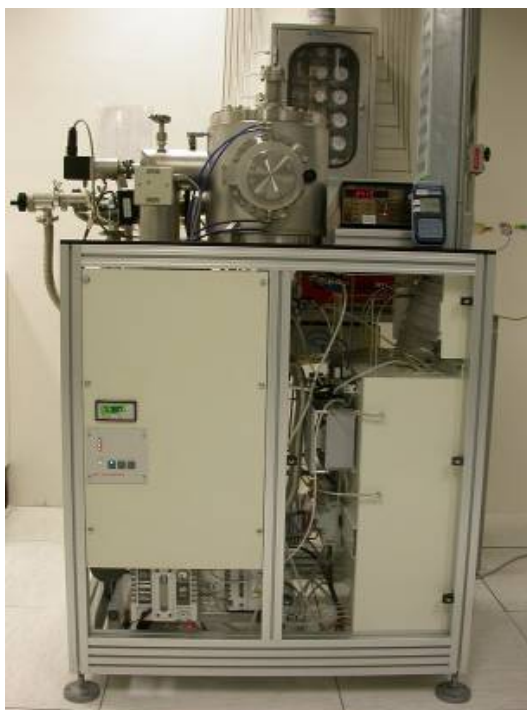
Figure 4.15. Photo of the Cold Walls Reactor.
