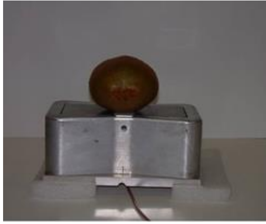
Fig. 9. Measurement of intact kiwifruit with a single-sided NMR sensor, (Capitani et al., 2010).
