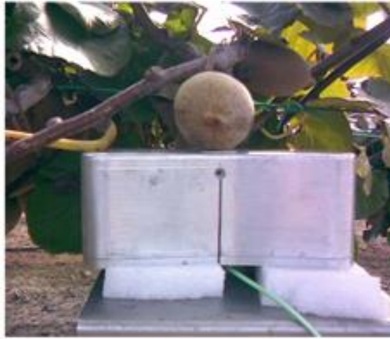
Fig. 11. Measurement in field on entire kiwifruit attached to the tree with a portable unilateral NMR instrument, (Capitani et al., 2013).
