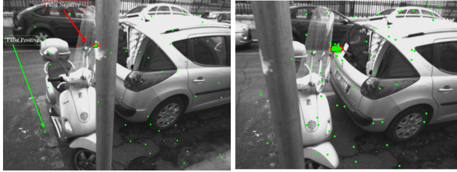
Figure 3.15: Results of features and classification validation for the outdoor experiment looking for parking fines . In red the PORs, and the coherent patches, in green the estimated point saliency, for the specific task.
