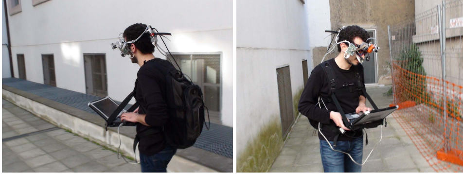
Figure 3.2: The Gaze Machine (GM) worn by the subject collecting PORs in an outdoor search task.
