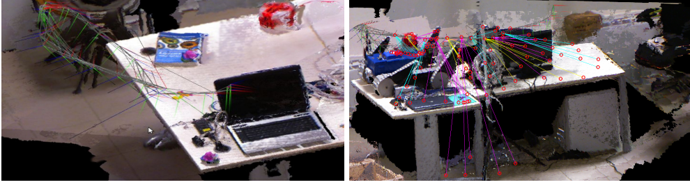
Figure 3.7: Head poses of the subject during the experiment searching for J , computed with the described localization algorithm, and the rays joining the head pose with the PORs (the red circles) projected on the scene point cloud. The lines represent, ideally, the intersection of the visual axes.
