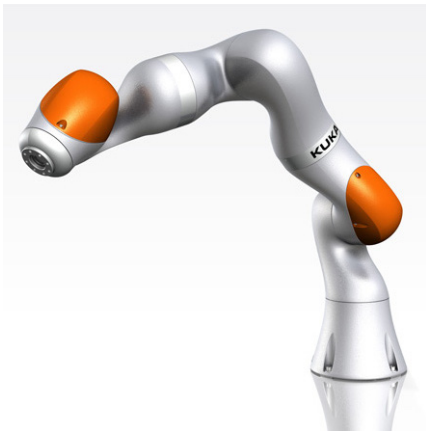
Figure 2 The KUKA LBR iiwa is a commercial lightweight manipulator with compliant joints. Image edited from [96].
