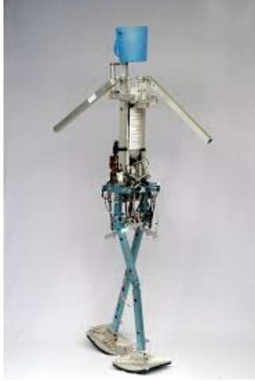
Figure 5.1 The passive humanoid robot Denise. Image edited from [88].
