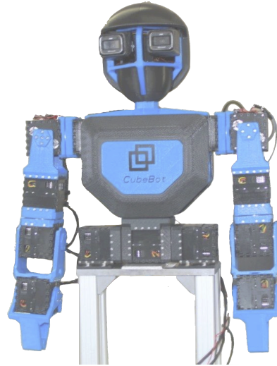
Figure 5 A small-sized humanoid built out of qbmove kits. Image edited from [97].
