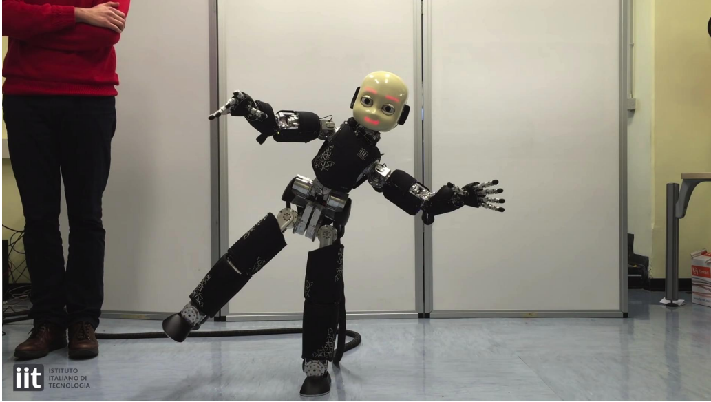
Figure 6.2 The iCub, seen here standing on a single foot, can be modeled as a fixed-base kinematic tree. Still frame from video associated to [59].
