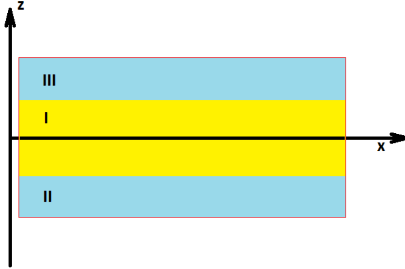
Figure 2.4. Geometry of a three-layer system consisting of a thin layer sandwiched between two infinite half spaces II and III.
